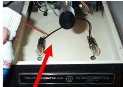
Blow out interior
