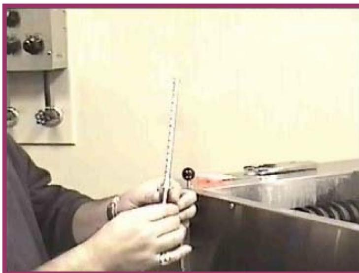
Hydrometers for micrographic chemistry may be obtained from many sources, below is one from VWR International.
