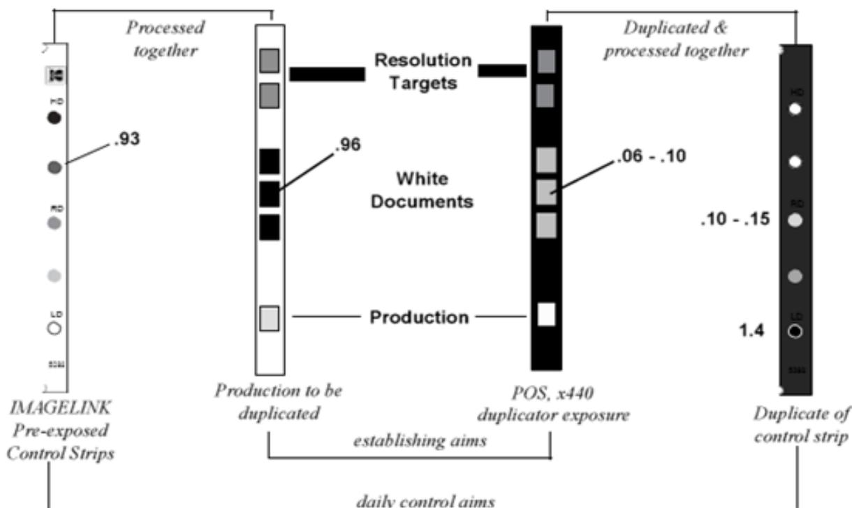
Figure 10: POS and x440 setup for establishing aims
